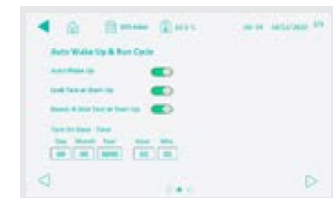
Auto-start function with a combination of wake up, Leak Test & Bowie & Dick/Warm-up Cycle
